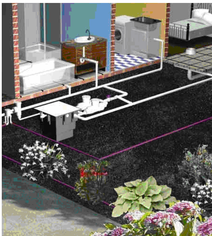
GRS SupaFlow System redirects greywater from the bathroom or laundry through a filter, which is then pumped into a subsurface dripper line.
