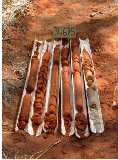
Deep soil cores used for soil moisture, chloride and matric potential measurements.
