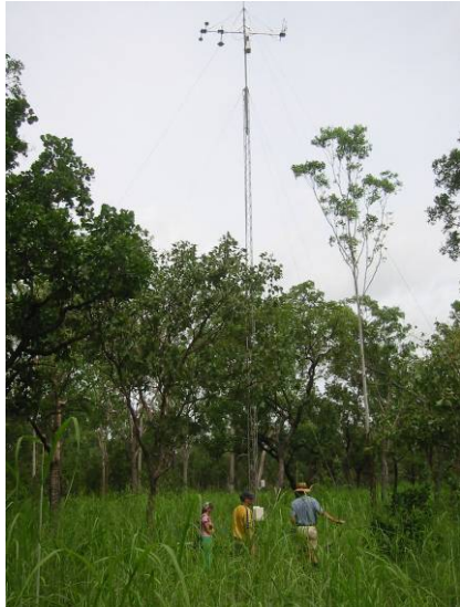
Eddy covariance tower at the uncleared site. It was used to determine evapotranspiration.
