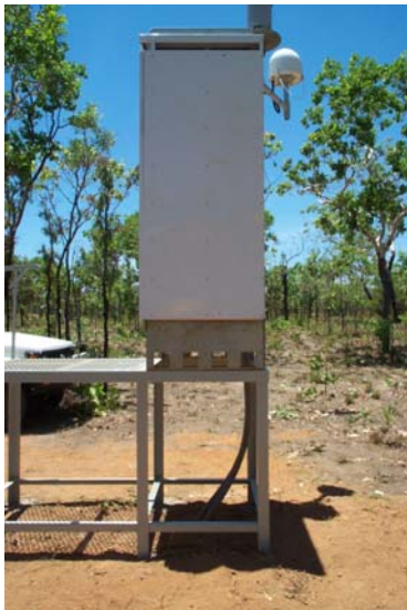
Photo 5 Instrumentation shelter and platform
