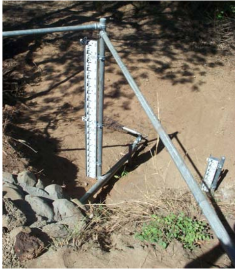
Photo 9 Example of Orifice and Turbidity Sensor end arrangements
