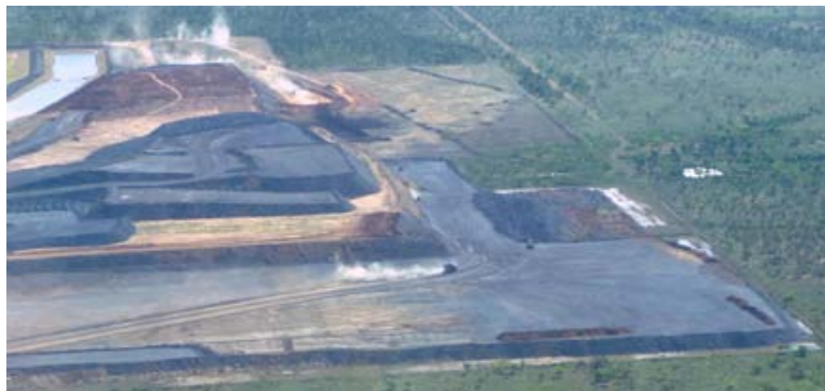
The clay layer that lines the base of the OEF is an essential part of the OEF design. The clay acts as a barrier to stop the migration of any acid production that may occur within the OEF waste rock. It is essential that the chemical and physical nature of the clay is tested before and after it is placed at the OEF to ensure its suitability. (May 2010).
