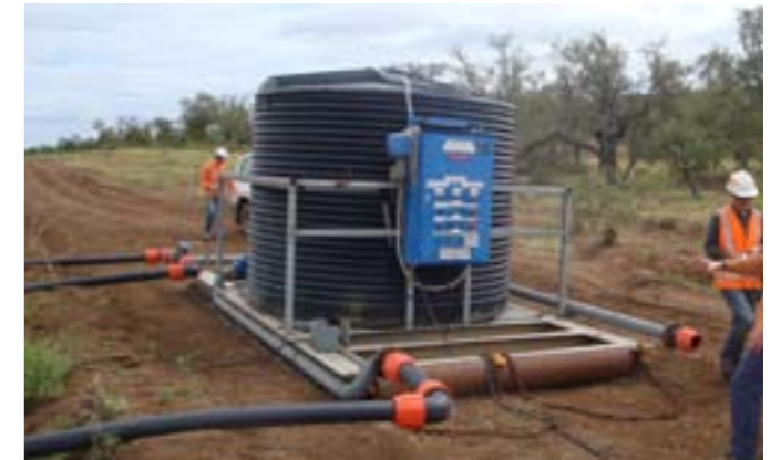
MRM have utilised a new irrigation sled to help establish vegetation along the McArthur River diversion channel over the 2010 dry season (May 2010).
