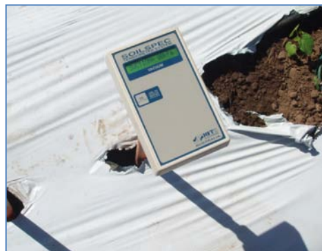
An electronic meter is used with tensiometers to measure soil water tension.
